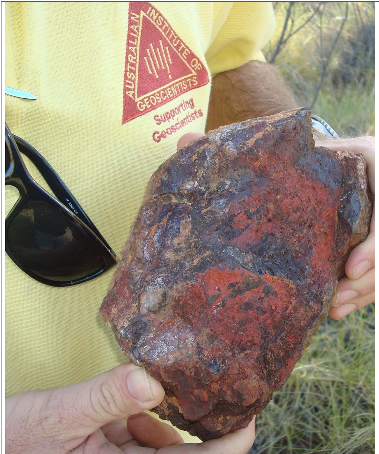
Plate 1. Prospecting utilising the handheld Niton XRF device has indicated elevated copper along strike 40m to the south east of GR-003. The host rock is Naraku Granite which has been brecciated by the copper mineralising fluid.
