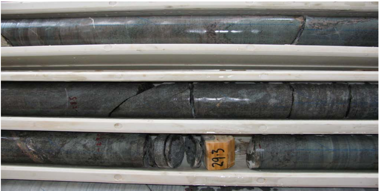
Photo 1: MKED003, 28.0 to 29.4 metres - Strong disseminated allanite-uraninite bands +calcite+pyrite in a diopside calc-silicate.
