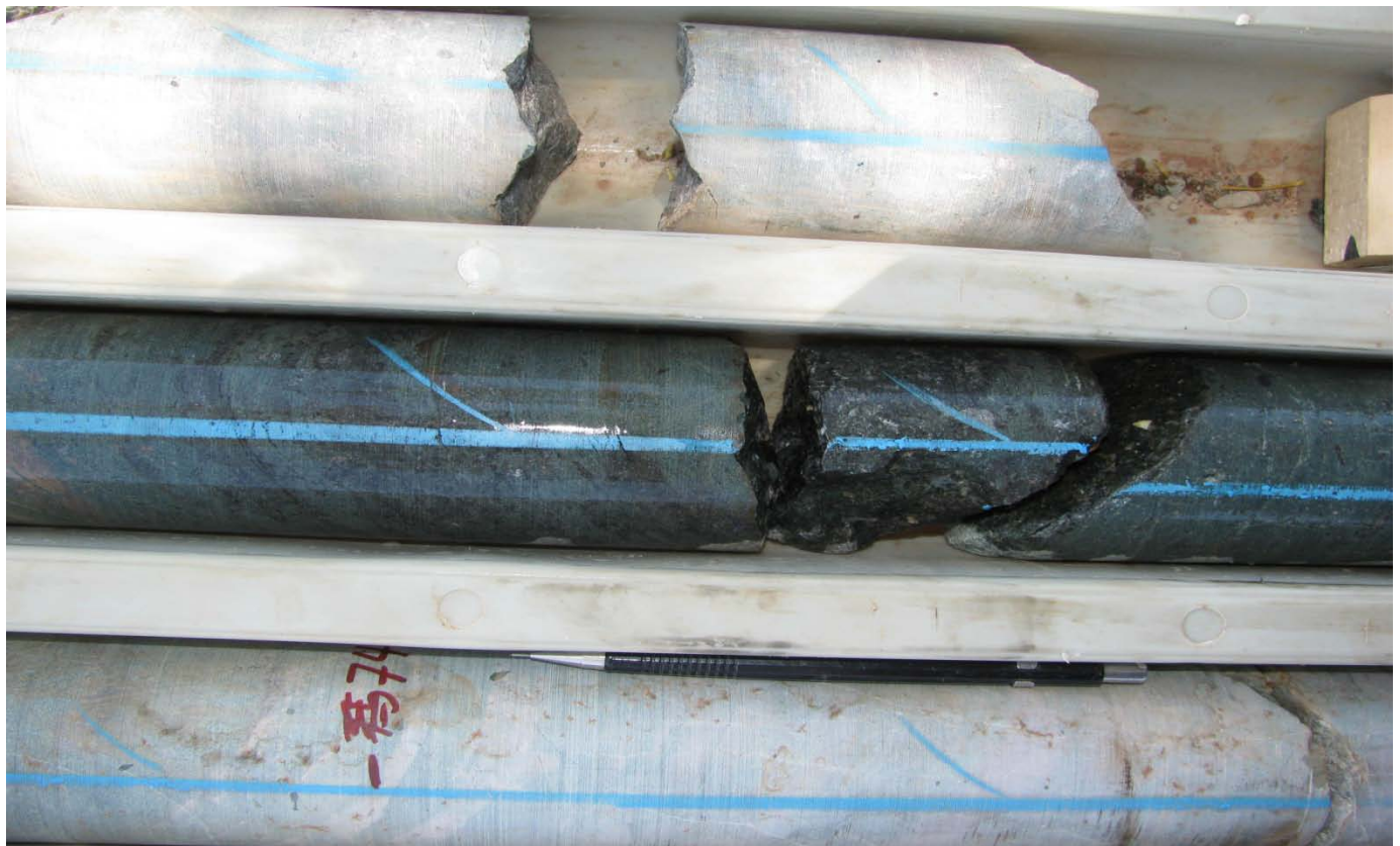
Photo 1: MKED_002, 74m - Strong disseminated allanite-uraninite bands +calcite+pyrite in a diopside calc-silicate.
