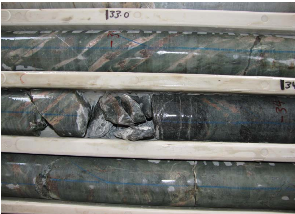
Photo 3: MKED001 - Mineralisation through broken, well-banded scapolite-diopside calc-silicate with garnetisation.
