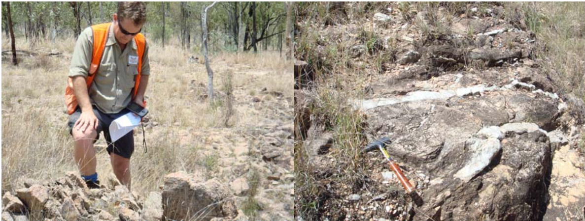
Figures 6 and 7 Mapping of auriferous quartz veins at The Gap prospect, Pentland.
