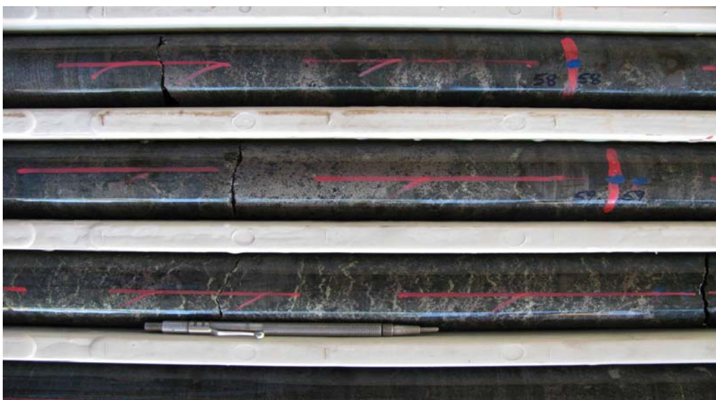
Photo 1: MKED004, ~57.00 to 60.00 metres - Strong fracture controlled pyrrhotite+pyrite+chalcopyrite mineralisation in a garnetite and diopside calc-silicate units. Assays returned for interval = 3m @ 1.04% copper, 361ppm cobalt and 0.09g/t gold .
